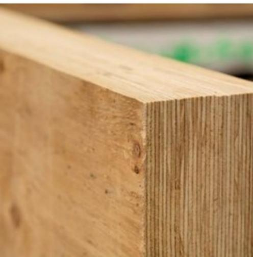
The systems of laser scanning and high-precision computerized mechanisms enable to recover natural inhomogeneities and defects from the sheets of veneer to produce the wooden material that is notable for its strength properties that are considerably better than the same of the solid (natural) wood.
